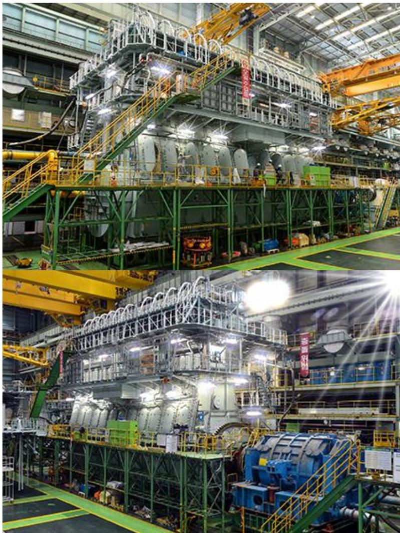
*Alternate views of the 11G95ME-C9.5 engine during its shop test in Korea (courtesy Doosan)*
