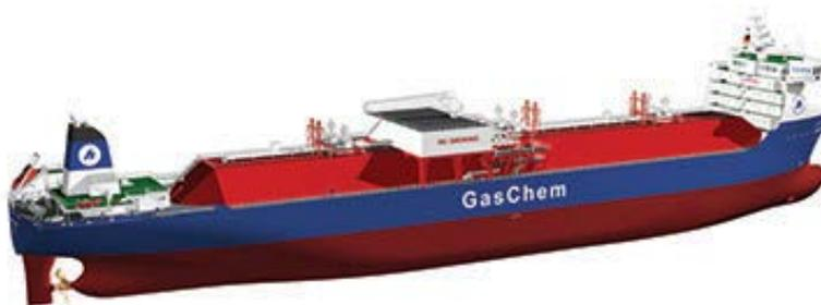
*Graphical rendering of a 36,000-m<sup>3</sup> GasChem ethane carrier featuring an MAN Diesel & Turbo Kappel propeller and rudder bulb, and an MM-Offshore EMPRESS rudder (courtesy Hartmann Reederei)*
