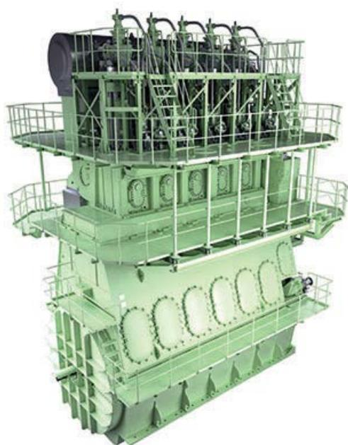
*Graphical rendering of the dual-fuel, gas-injection MAN B&W 5G70ME-GI engine*
