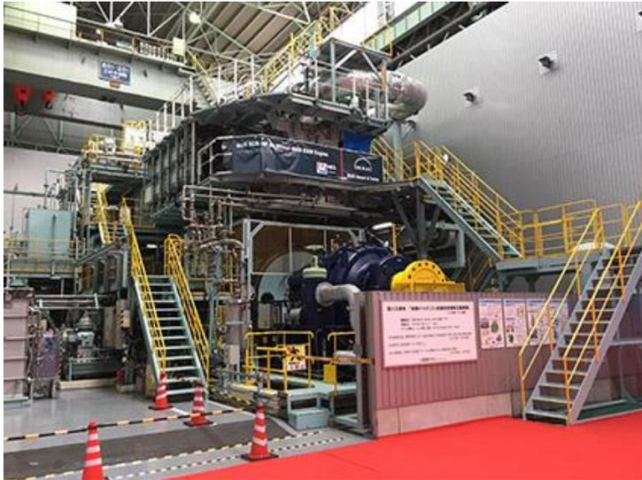
*The Mitsui-MAN B&W 4S50ME-T9 test engine hosting the new MAN SCR-HP technology*
