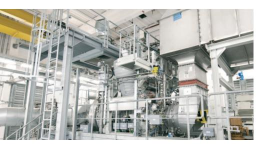
MAN PrimeServ provides a direct drive concept to modernize the positioning of the inlet guide vanes, the fuel control valve and the dilution air flaps.
